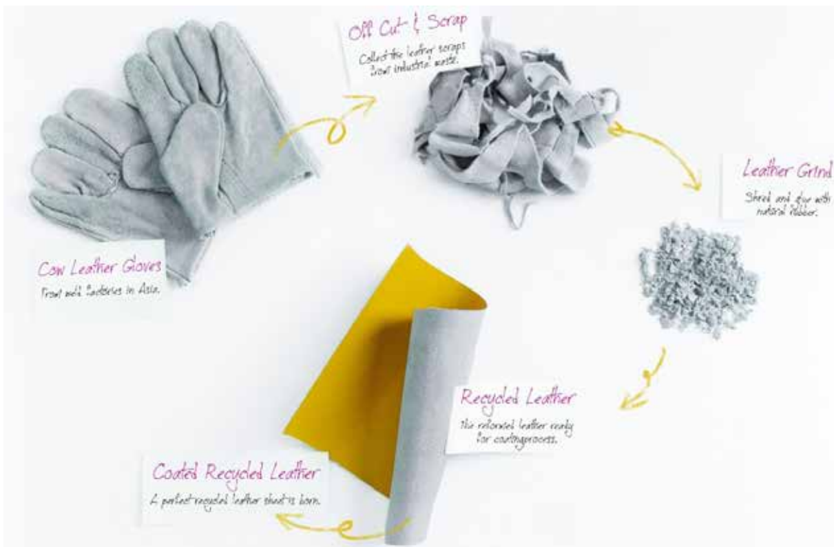
IMAGE: The recycling process, image supplied by one of our recycled leather suppliers, Recyc Leather™ who use a natural rubber binder
